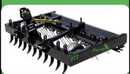
The MINI DragNfly has an open cage roller on the front, next there is three rows of tines that work like fingers to mix and spread the surface keeping the footing from clumping, giving an ultimate mixing effect of the surface. This drag is designed to mix the surface only. This drag cannot dig, working great for shallow footing surfaces. It can be pulled behind ATV, golfcart etc.or small compact tractor. Sizes D60",D72",D84"D96"
