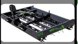
The MINI DragNfly has an open cage roller on the front, next there is three rows of tines that work like fingers to mix and spread the surface keeping the footing from clumping, giving an ultimate mixing effect of the surface. This drag is designed to mix the surface only. This drag cannot dig, working great for shallow footing surfaces. It can be pulled behind ATV, golfcart etc, or small compact tractor.
